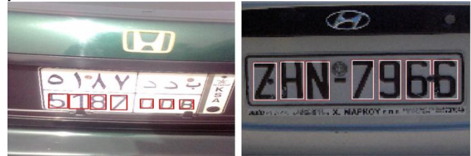
Fig. 17. Examples for locating symbols touching the digit's bounding box (digit '1' in (a)) and touching each other (last two digits in (b)).
